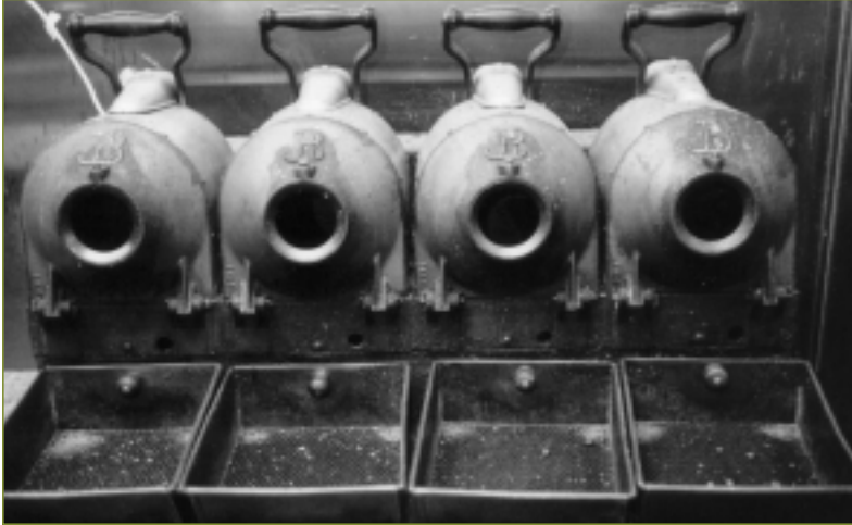
Not far from the grinders sat a row of Jabez-Burns sample roasting drums...
